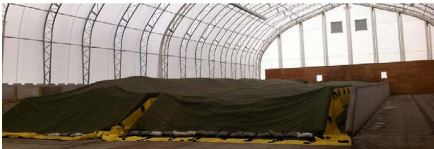
Photo 15: Salish Soils – Gore Cover Composting System
